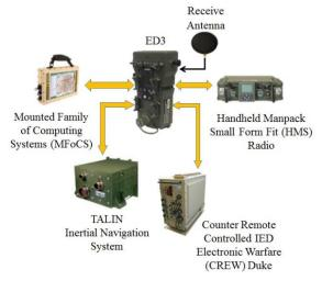
Figure 4 ED3 Notional Installation
